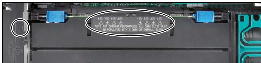
Figure 36: Example: Diagnostic LEDs on memory board B
